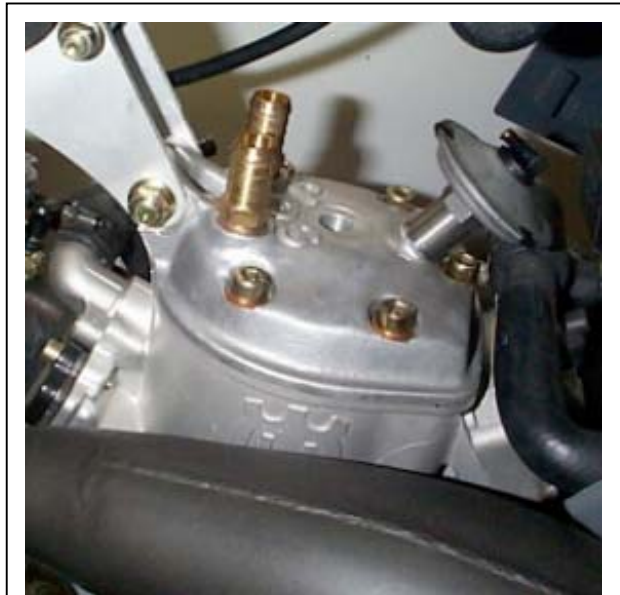
Step 2: Completing head installation – Tighten head bolts to in manner presented above, fit and tighten decompressor valve to head ensuring the outlet pipe faces directly backwards (towards the carburettor). Tighten head mounting plates to manufacturers spec., fit and tighten radiator hoses, spark plug, refill radiator, check for leaks.
