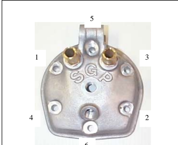
Cylinder head tightening sequence. Tighten cylinder head bolts firmly in sequence presented above to seat orings, then proceed to torque bolts in the same sequence to 20Nm(15ft/lb).
