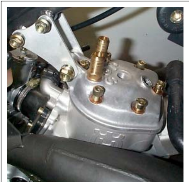
Step 1: After removal of standard cylinder head clean surface of barrel ensuring no foreign matter falls into combustion chamber or water jackets. LIGHTLY grease head orings with rubber grease and replace using new ones if necessary. Fit decomp head, head mounting plates and all nuts and bolts loosely – do not tighten at this stage.
